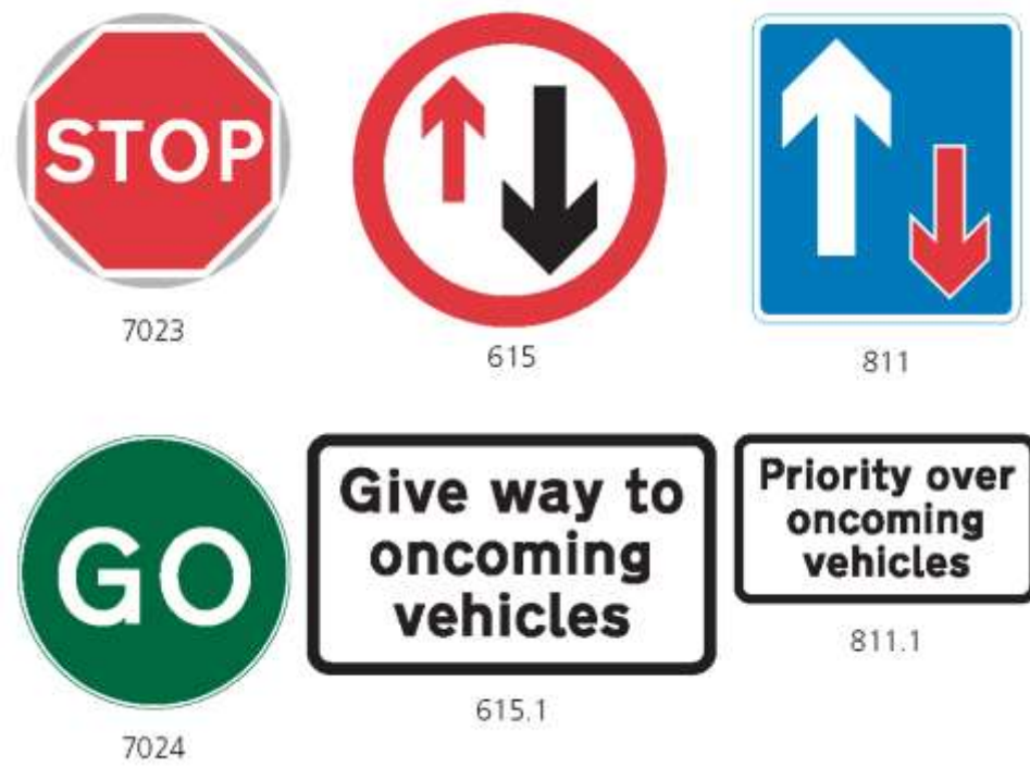
Figure 3.5: Manually Operated Stop/Go Signs and Priority Signs.
